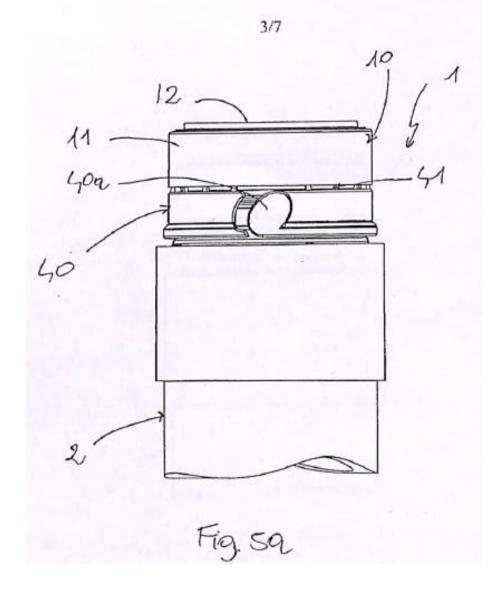
53. In this figure 5a above, it is seen that reference numeral 10 is the container cap, reference numeral 40a is the second tear off seal which upon being torn, separates the perforation from the cap thereby allowing the user to open the container. Upon the second tear off tab being opened, the depiction would be as under:
